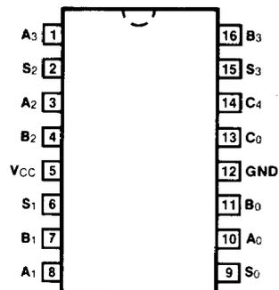
**DESCRIPTION** — The '83A high speed 4-bit binary full adders with internal carry lookahead accept two 4-bit binary words ( $A_0 - A_3$ ,  $B_0 - B_3$ ) and a Carry input ( $C_0$ ). They generate the binary Sum outputs ( $S_0 - S_3$ ) and the Carry output ( $C_4$ ) from the most significant bit. They operate with either HIGH or active LOW operands (positive or negative logic). The '283 is recommended for new designs since it features standard corner power pins.
