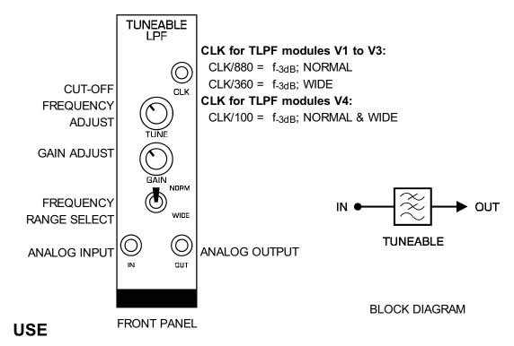
This lowpass filter has an elliptic filter characteristic. The stopband attenuation is typically 50dB and passband ripple is approximately 0.5dB.
