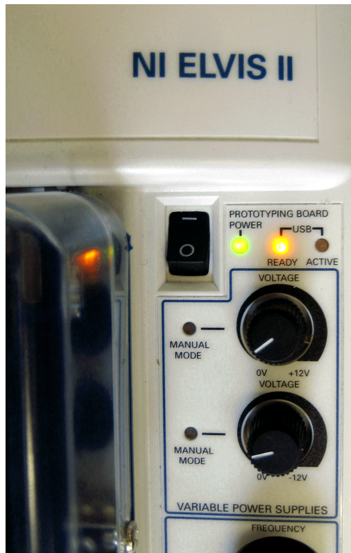
Figure 6.7: Ready and Power LEDs on NI ELVIS II
